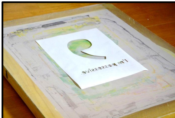
STENCIL FACE DOWN ON SIDE B OF SCREEN
