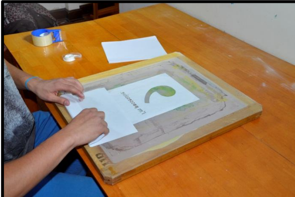
PRINTING PAPER USED TO COVER REMAINDER OF SCREEN
